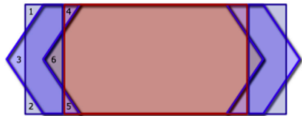
Fig. 5 Overlapping of the layouts of the Diamond and Rectangular MOSFETs in order to verify if their total die areas are similar.
