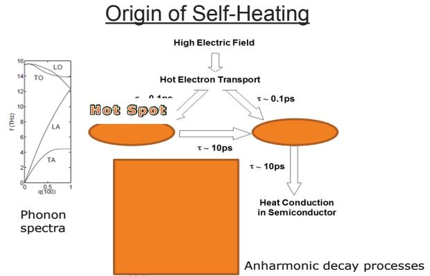
Figure 2. Transfer of energy from the electron system to the acoustic and optical phonon baths.
