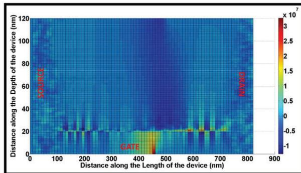
Figure 8. Difference between the vertical component of electric field in the simulation including self-heating effects and excluding the same.
