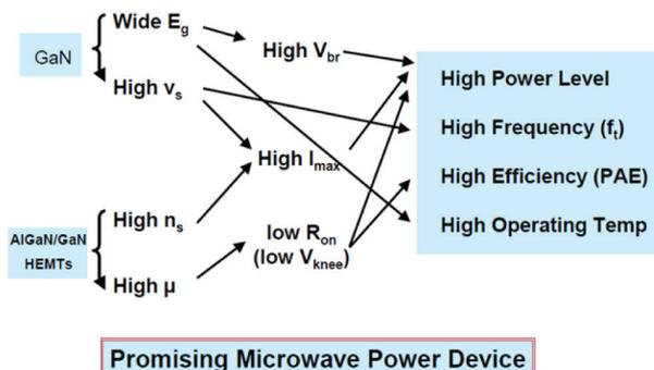
Figure 1. Applications for GaN bulk materials and AlGaIn/GaN HEMTs.
