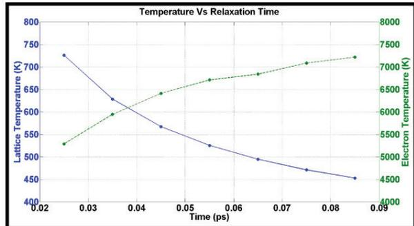
Figure 7 . Maximum Lattice and Electron Temperature vs. Phonon relaxation time ( $V_G=0V$  and  $V_D=8V$ ).
