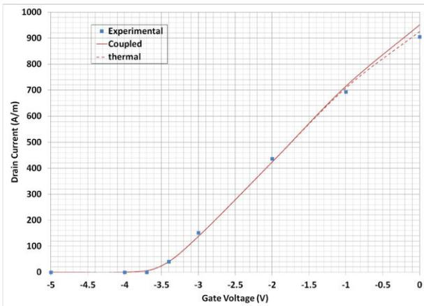
**Figure 9.** Simulated transfer characteristic of the device for  $V_D=5V$ . Also shown here are available experimental data.
