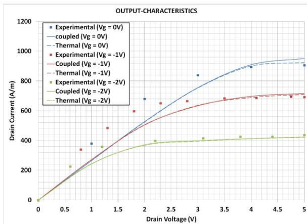
**Figure 10.** Simulated output characteristics of the device from Fig. 4 together with experimental data (symbols)
