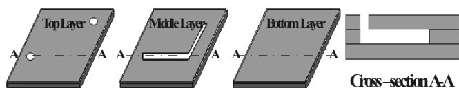
Fig. 2. Micro-channel implementation using LTCC
