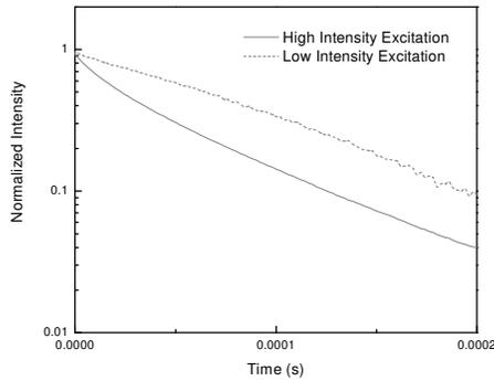
Fig. 2: Emission lifetime for the lead fluoroborate glasses doped with 1.75 w% of  $Nd_2O_3$  ( ${}^4F_{3/2} \rightarrow {}^4I_{11/2}$  transition).
