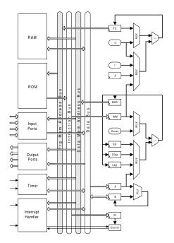
Figure 1. The FemtoJava Micro Architecture
