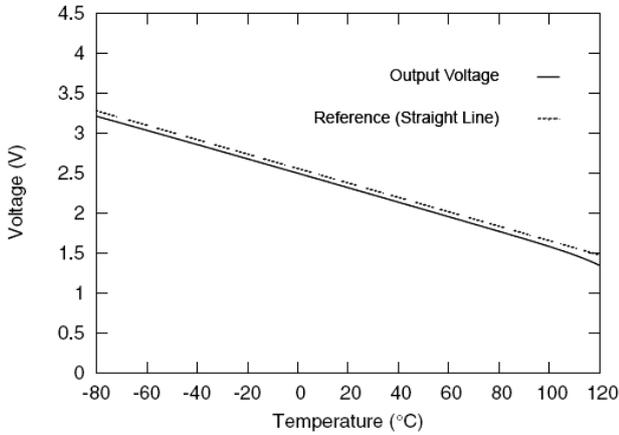
Fig 2. Output Voltage as a function of the Temperature
