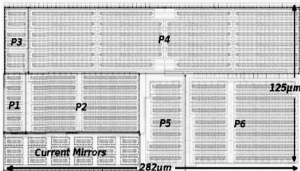
Fig 6. Layout of the implemented sensor
