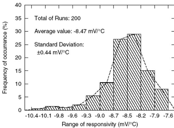
Fig 3. Histogram of Responsivity affected by variations on transistors sizes, using Monte Carlo Analysis
