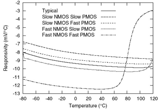
Fig 4. Responsivity for Typical and Corner Cases
