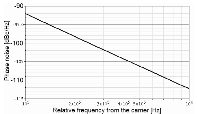
Figure 4: Post-layout simulated phase noise.
