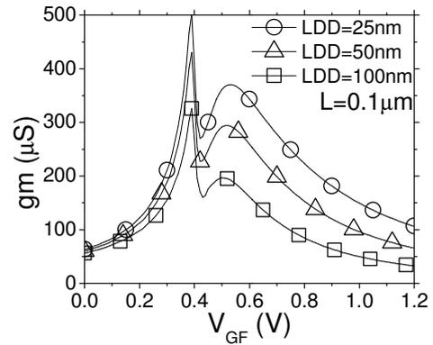
Figure 5: Transconductance as a function of gate voltage for different LDD lengths and channel length equal to  $0.1\mu m$ .
