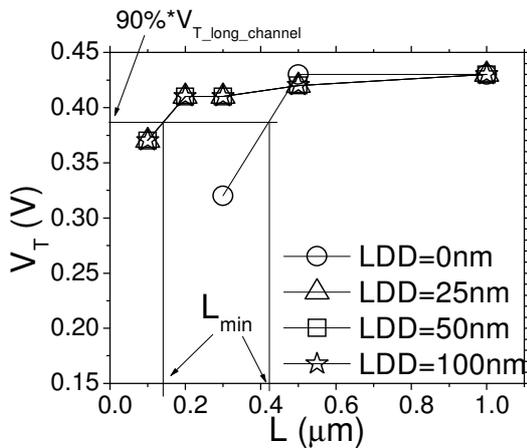
**Figure 7: Threshold voltage as a function of channel length for different LDD lengths allowing the extraction of the  $L_{min}$  value.**
