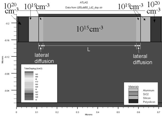
Figure 3: Doping concentration in SOI LDD MOSFET structure obtained by simulations.
