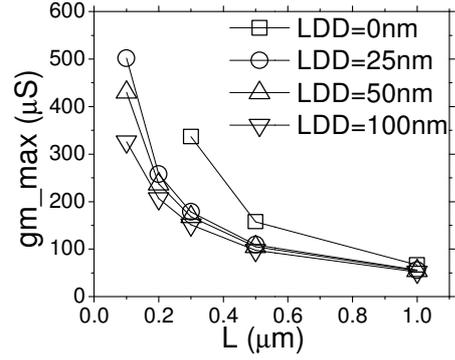
Figure 4: Maximum transconductance versus channel length for different LDD length.
