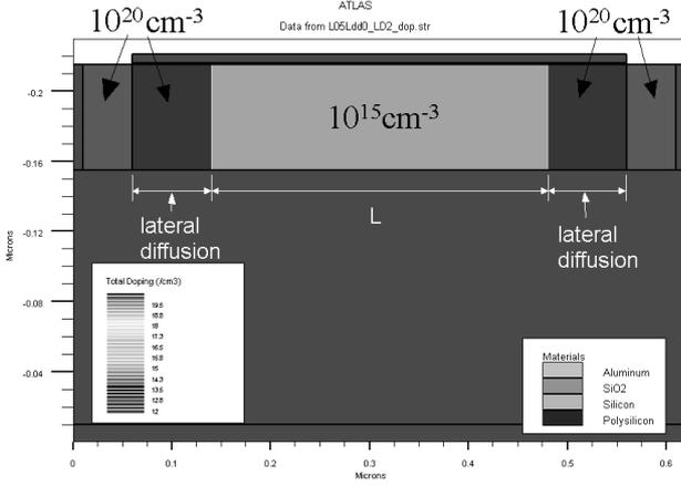
Figure 2: Doping concentration of SOI MOSFET structure without using LDD regions obtained by simulations.
