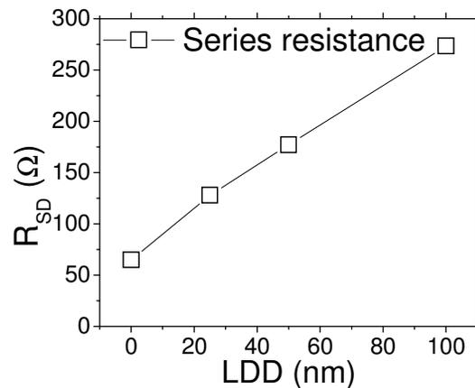
**Figure 8: Series resistance as a function of LDD length.**
