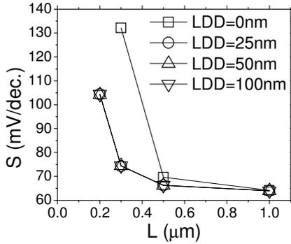
**Figure 6: Subthreshold slope versus channel length for different LDD lengths.**
