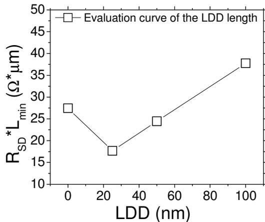
Figure 9: Curve to evaluate the optimum LDD length value (series resistance multiplied with the minimum channel length versus LDD length).
