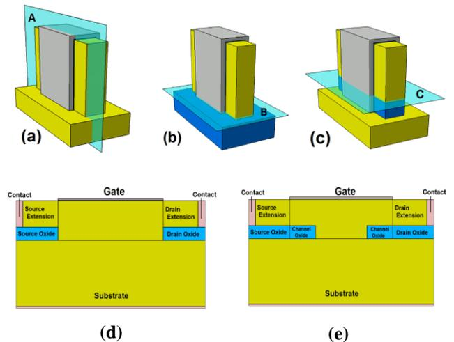
**Fig. 1. Simulated structures and peculiarities. (a) Bulk FinFET; (b) SOI FinFET/ Pi Gate FinFET; (c) DSOI/M-DSOI FinFET; (d) DSOI vertical plane A; (e) M-DSOI vertical plane A.**
