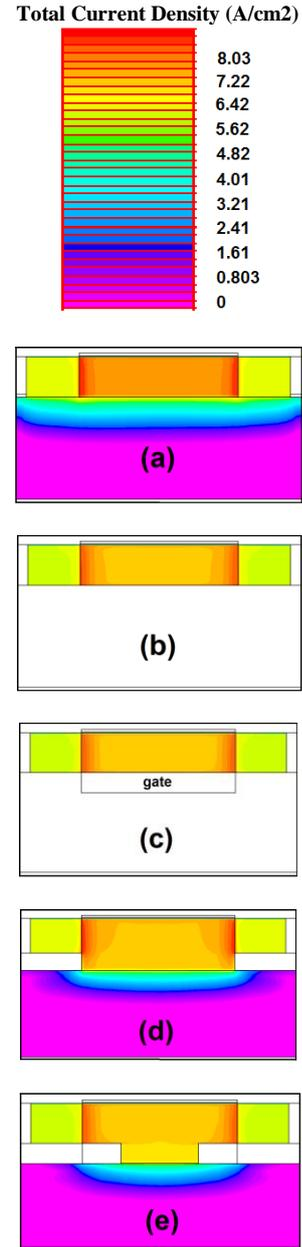
**Fig. 5. Current density for five transistors using plane A. (a) Bulk FinFET; (b) SOI FinFET; (c) Pi Gate SOI FinFET; (d) DSOI FinFET; (e) M-DSOI FinFET.**
