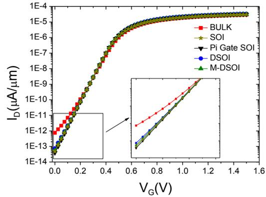
**Fig. 3. Subthreshold Slope (SS) for Bulk, SOI, Pi Gate SOI, DSOI and M-DSOI FinFET devices.**
