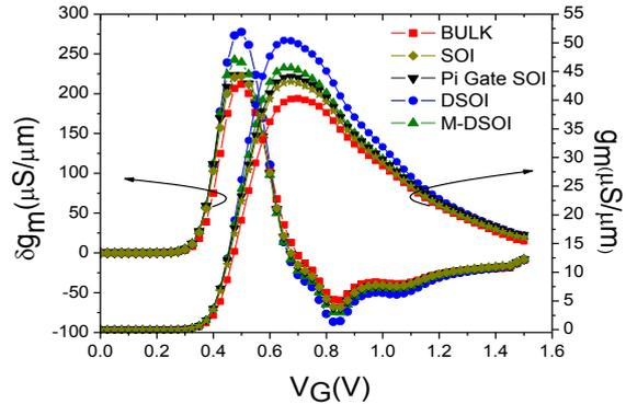
**Fig. 4. Second  $g_m$  derivate and  $g_m$  for BULK, DSOI, M-DSOI, Pi Gate SOI and SOI FinFET devices.**
