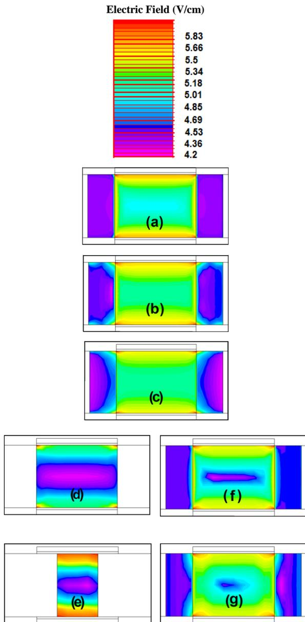
**Fig. 6. Electric field distribution for five transistors using plane B: (a) Bulk FinFET; SOI FinFET (b); Pi Gate SOI (c); (d) DSOI FinFET; (e) M-DSOI FinFET. Electric field distribution for five transistors using plane C: (f) DSOI FinFET; (g) M-DSOI FinFET.**
