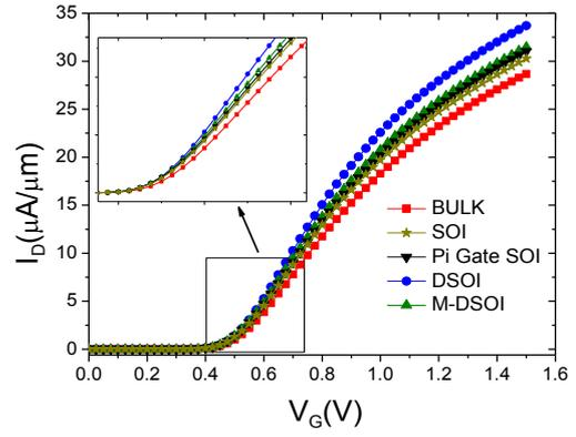
**Fig. 2.  $I_D \times V_G$  curve for Bulk, SOI, DSOI, Pi Gate SOI, and M-DSOI FinFET devices.**
