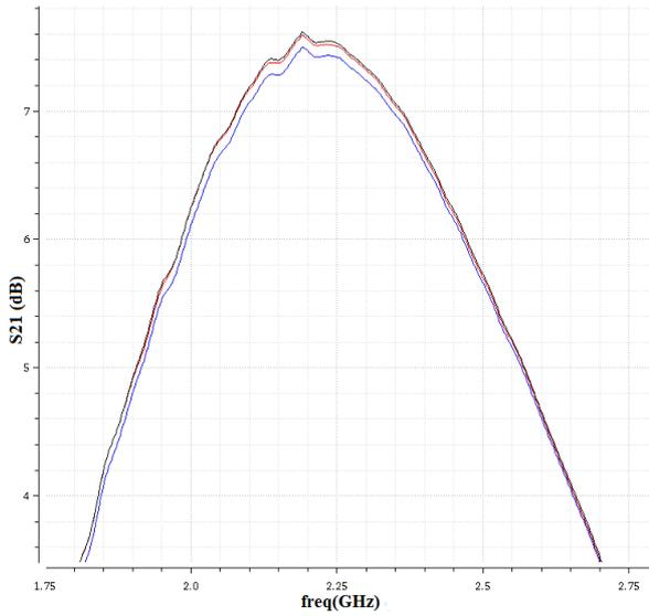
Fig.6. S21 for three LNA samples.
