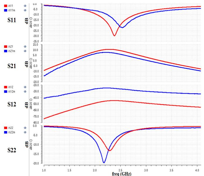
Fig. 5. Post-layout simulations (red) and final LNA (blue) S-parameters.
