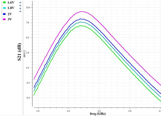
Fig. 7. S21 under different supply voltages: 1.6 V (green), 1.8 V (light blue), 2 V (blue) and 3 V (pink).
