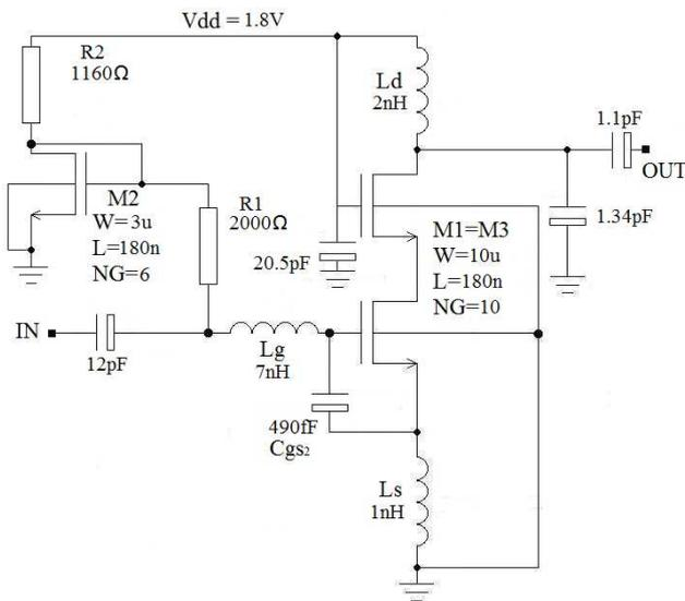
Fig.3. LNA Schematic.
