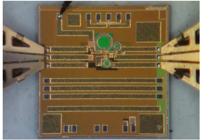
Fig. 4. Microphotography of the LNA.
