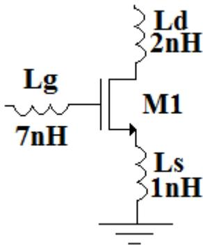
Fig. 2. Circuit with inductors of the technology.
