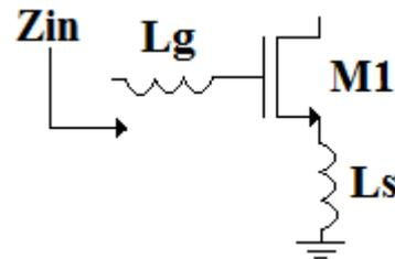
Fig. 1. Inductive source degeneration topology.
