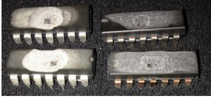
Fig. 1 - Detail of the Integrated Circuit CD4007 used on the experiments, after the removal of the epoxy layer.
