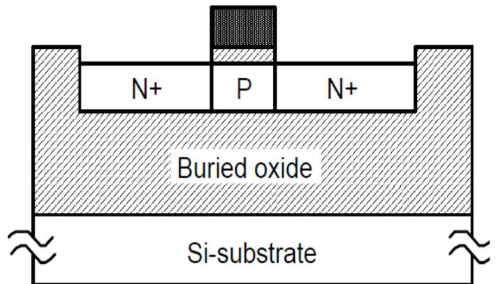
Fig. 1. The SOI transistor. Source: [5]
