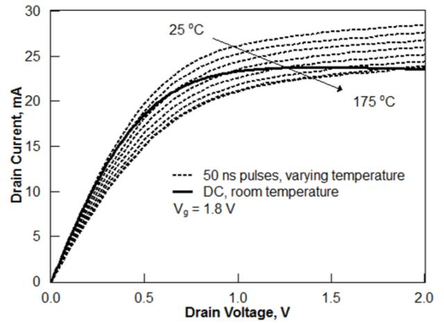
Fig. 2. Drain current versus drain voltage varying temperature with voltage pulses applied to the gate. Source: [3].
