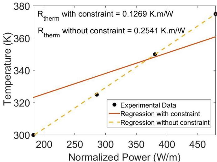
Fig. 5. Obtaining the thermal resistance with and without the theoretical constraint
