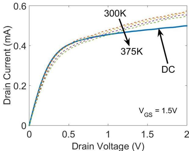
Fig. 4. Drain current versus drain voltage considering DC (room temperature) and pulsed measurements (varying temperature) for a UTBB device
