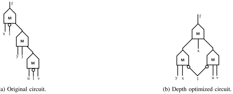
Fig. 2: Majority circuits described by Equation 1.
