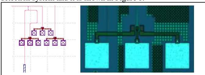
Fig. 1. Circuit layout. Micrograph of on-chip Ge photodetector device used.
