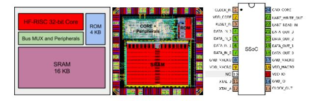
The first tests were conducted to certify that the clock, reset and UART were working properly using a breadboard. After that, we developed a simple (Arduino-like) platform to validate all of the SSoC blocks through a simple C library<sup>1</sup> and demos. All planned features are working well except for minor problems caused by the first reset and the system power-up sequence, due to
