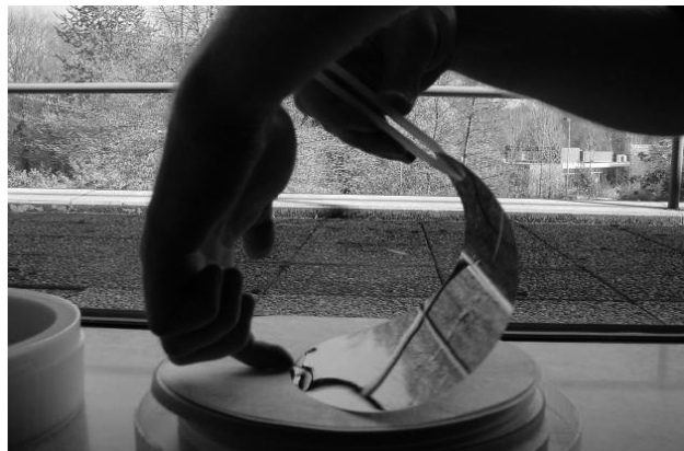
Figure 2. a 200 mm wafer after thinning down to 50 \mu\text{m} becomes flexible.
