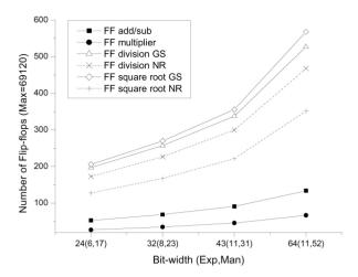
Figure 4. Flip-flops consumption
