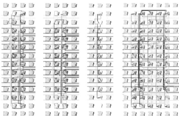
**Figure 10.** Different reconfigurable instructions: barrel shifter, saturation add/subb, 64 input XOR gate, '1' bit counter (from left to right).
