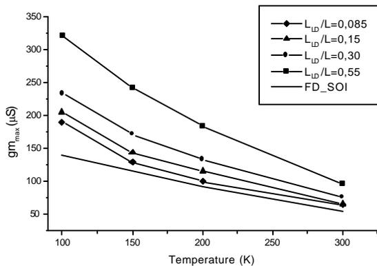
Figure 3: Maximum transconductance versus temperature ( $gm \times T$ ) for several  $L_{LD}/L$
