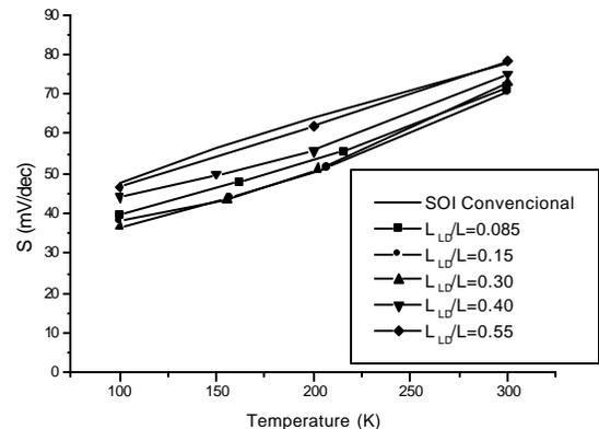
Figure 2: Subthreshold versus Temperature ( $S \times T$ ) for several  $L_{LD}/L$  rates.
