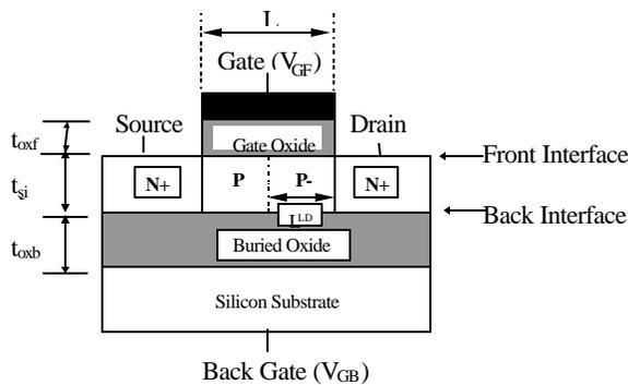
Figure 1: GC-SOI nMOSFET structure
