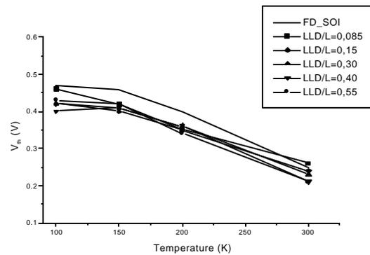
Figure 4a: Threshold voltage versus Temperature.
