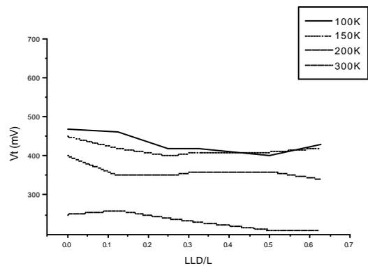
Figure 4b: Threshold voltage versus several  $L_{LD}/L$
