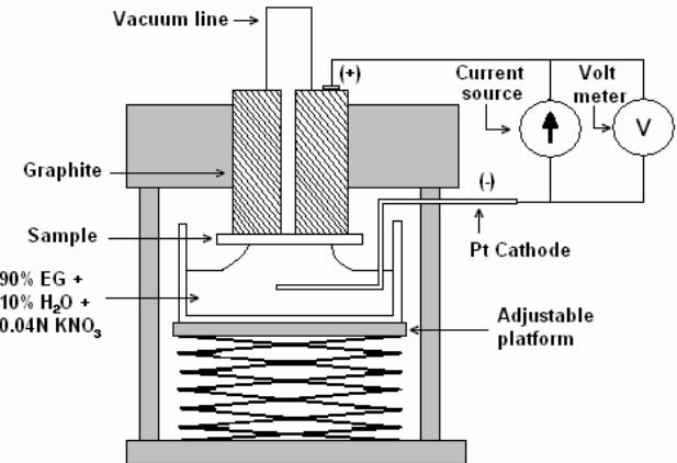
Figure 2. Anodic oxidation equipment used for charge carrier profile measurements.
