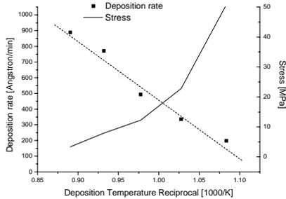
**Figure 1: Stress by scan profiler and deposition rate dependency on deposition temperature.**
