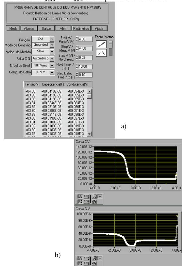
Figure 1 – Main Frontal Panel with a) the measurement variables input and the table with the results and b) the graphical part.
