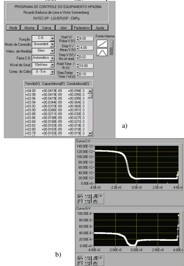
Figure 1 – Main Frontal Panel with a) the measurement variables input and the table with the results and b) the graphical part.
