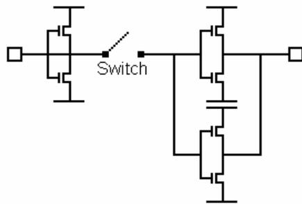
**Figure 01 – Two Unity Gain Current Buffer Switched Current Cell**
