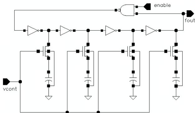
Figure 1: Schematic of vco\_0813.
