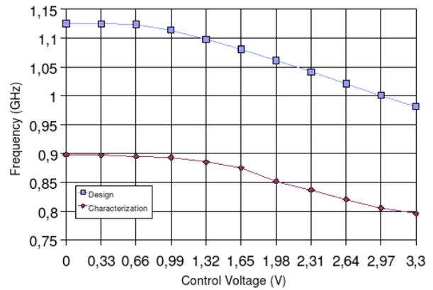
Figure 7: Simulated and measured characteristic of vco\_0903.
