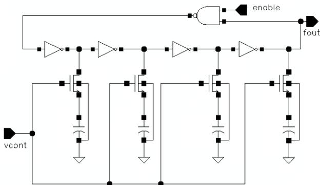
Figure 1: Schematic of vco\_0813.
