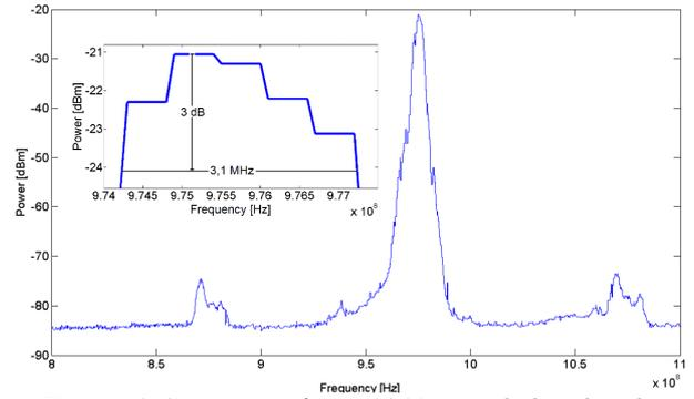
Figure 6: Spectrum of vco\_0813 in wide band and in narrow band showing the peak.
