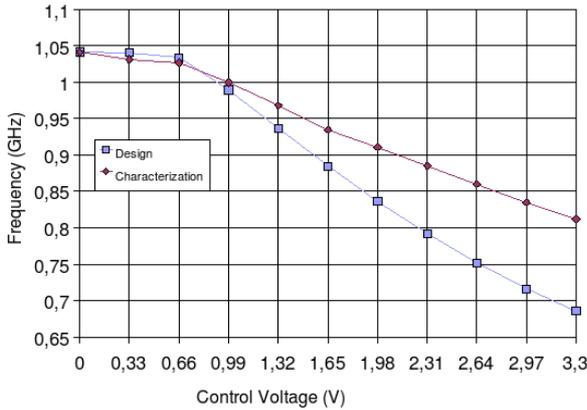
Figure 5: Simulated and measured characteristic of vco\_0813.
