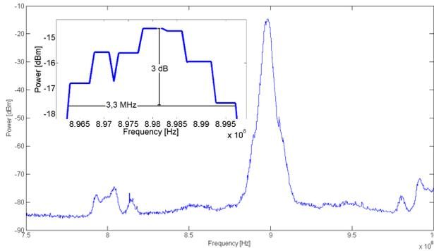
Figure 8: Spectrum of vco\_0903 in wide band and in narrow band showing the peak.
