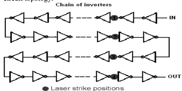
Fig. 1 – Chain of inverters showing the Laser pulse strike positions
