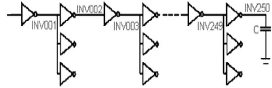
Fig. 2 – Schematic description of the chain of inverters with (a) a standard design, or (b) with every other inverter triplicate to simulate the load of more complex designs
