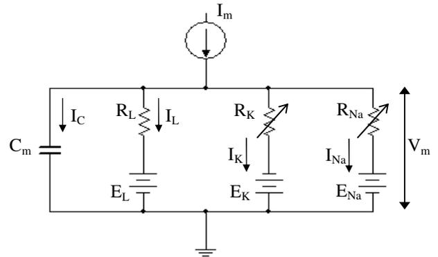
Figure 1 - Schematic diagram of the Hodgkin-Huxley circuit. The subscript  $m$  and  $L$  stands for membrane and leakage respectively. This last subscript is due to the leakage current that model the effect of the ions that are not being explicitly considered within the dynamics of the cell membrane depolarization and repolarization.
