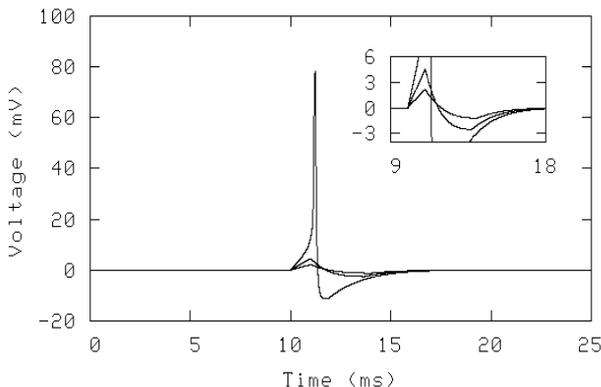
Figure 6 - A current of 10  $\mu$ A generates a spike about 80 mV. On the other hand, currents of 2.5  $\mu$ A and 5  $\mu$ A are insufficiently strong to generate an action potential, then, there is merely a slight voltage variation above the resting potential of the membrane (see insert in the top right of the figure).
