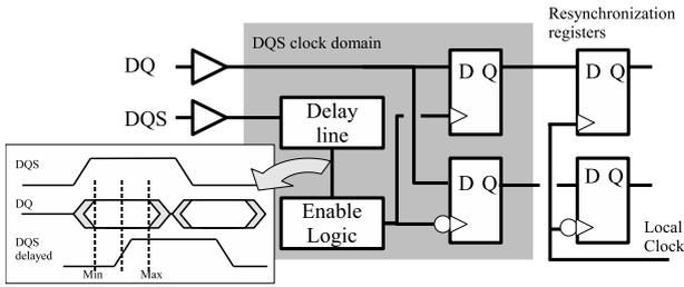
Figure 4. Circuit topology to capture the data read.
