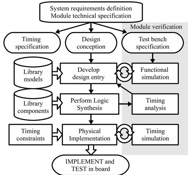
Figure 1. IP module design flow for FPGA.
