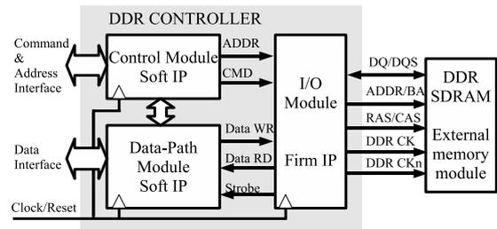
Figure 3. DDR controller block diagram.
