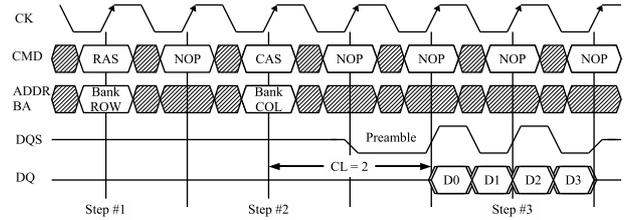
Figure 2. Timing diagram of reading data from DDR memory with CAS latency 2 and burst length 4.
