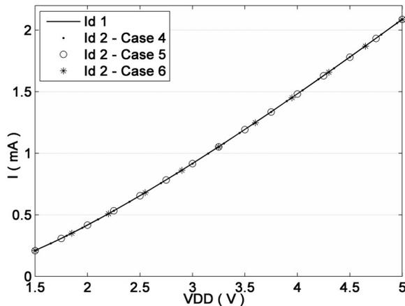
Fig. 6. Id2 current for cases 4, 5 and 6, using EKV models.
