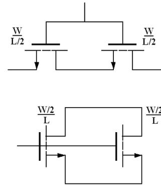
Fig. 1. Series and parallel association of MOSFET's.
