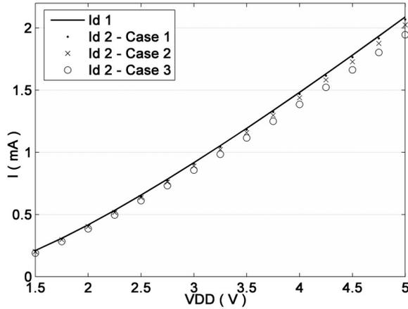
Fig. 5. Id2 current for cases 1, 2 and 3, using EKV models.
