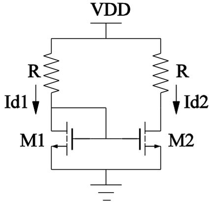
Fig. 2. MOSFET current mirror schematic diagram.
