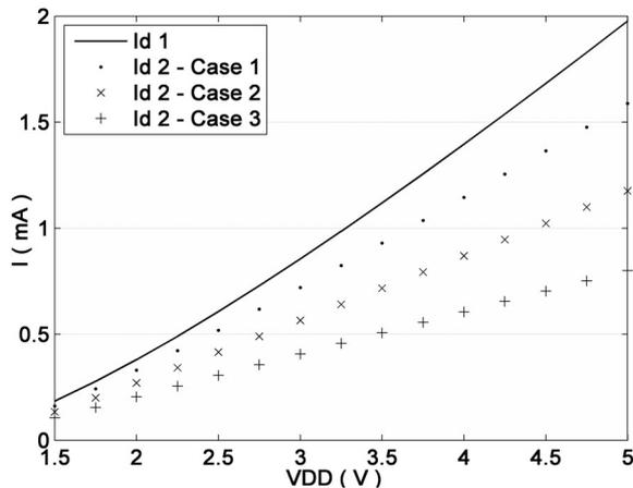
Fig. 3.  $I_{d2}$  current for cases 1, 2 and 3, using BSIM3v3 models.
