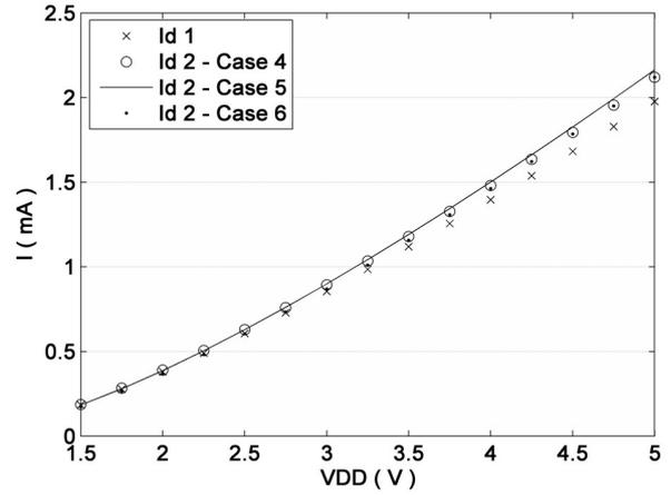
Fig. 4.  $I_{d2}$  current for cases 4, 5 and 6, using BSIM3v3 models.
