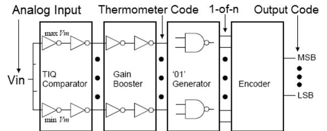
Fig. 1. Block diagram of the TIQ ADC
