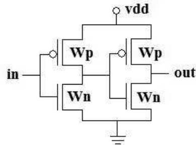
Fig. 2. TIQ comparator schematic
