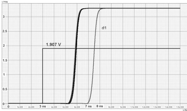
Fig. 7. Delay analysis ([d3,d2,d1,d0] x time) showing a maximal 4,5 ns delay for the bit d1.
