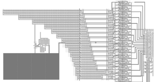
Fig. 6. The 4 bit TIQ Flash ADC generated layout, with sampling circuit.  $1143 \times 627 \lambda^2 = 0.0448 \text{ mm}^2$
