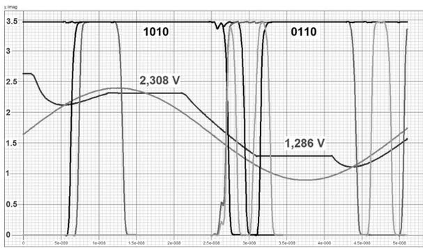
Fig. 9. A Transient analysis ([d3,d2,d1,d0] x time) showing an example of conversion using the track-and-hold circuit designed.  $f_{\text{sgn}} = 20\ \text{MHz}$ ,  $F_s = 50\ \text{MHz}$ , amplitude = 1.5 Vpp
