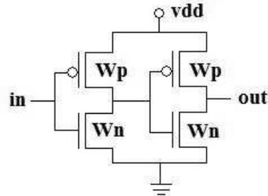
Fig. 2. TIQ comparator schematic
