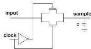
Fig. 5. Track-and-hold schematic
