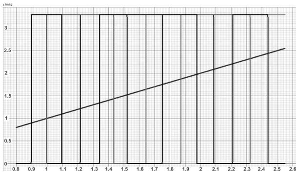
Fig. 8. A DC analysis ([d3,d2,d1,d0] x Vin) showing the threshold voltages for a DC input from 0.8 V to 2.55 V
