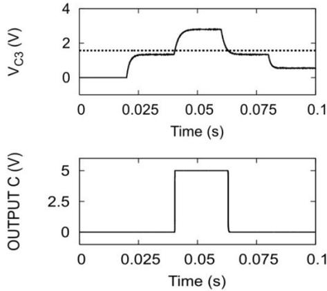
Figure 11: For a transient simulation of 0.1s, the voltage across the capacitor  $C_3$  and the threshold value of approximately 1.6V is shown in the upper graphic. The lower graphic is the AND logic result of this implementation.
