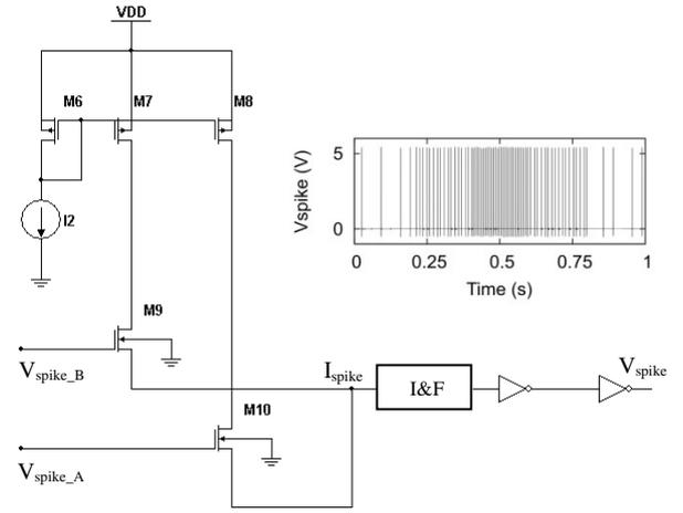
Figure 9: Block 1 circuit schematic and its output during a transient simulation with the same stimuli used in Figure 7: the signal  $V_{spike}$ .
