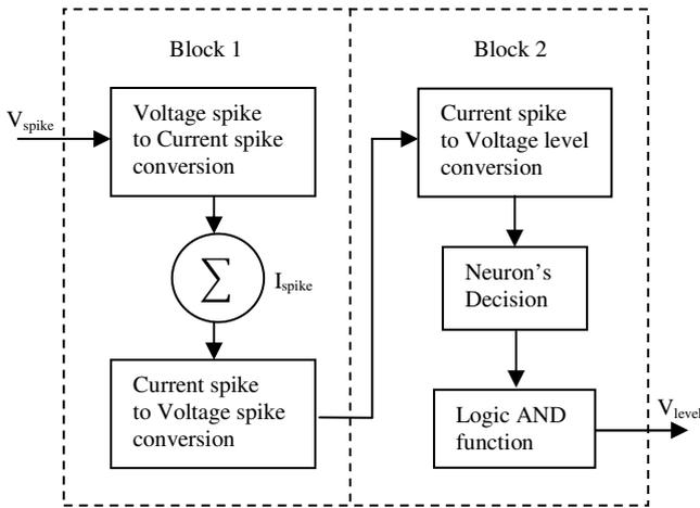
Figure 8: Neuron Block and its minor blocks 1 and 2.
