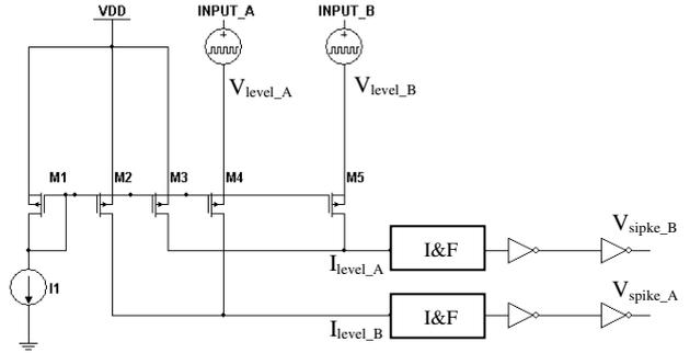
Figure 6: Schematic of the input conversion block circuit.
