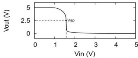
Figure 12: Inverter 1 transfer characteristic. The voltage switching point is 1.5686V.
