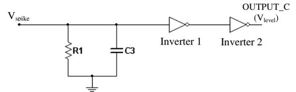
Figure 10: Block 2 circuit schematic, where  $R1=100k\Omega$  and  $C3=0.1\mu F$ .
