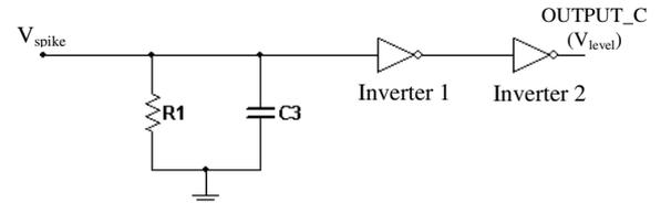
Figure 10: Block 2 circuit schematic, where  $R1=100k\Omega$  and  $C3=0.1\mu F$ .
