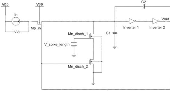
Figure 3: Schematic of the integrate-and-fire neuron electronic circuit. The value of  $V_{spike\_length}$  is equal to  $VDD$ .
