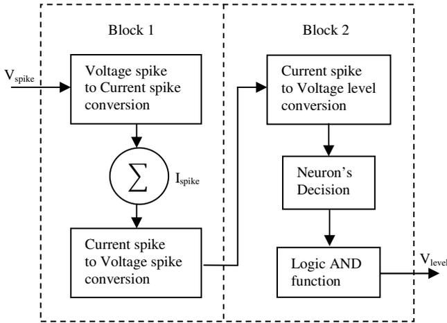
Figure 8: Neuron Block and its minor blocks 1 and 2.
