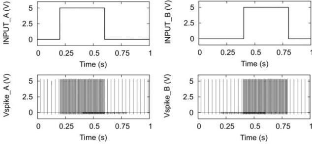
Figure 7: Voltage signals representing the binary inputs A and B as well as the voltage spikes representing the outputs  $V_{spike\_A}$  and  $V_{spike\_B}$ .
