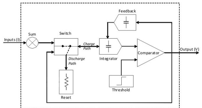
Figure 2: Integrate-and-fire neuron model. The integrator block is formed by a capacitor as well as the feedback block. The switch and reset blocks are implemented with transistors.
