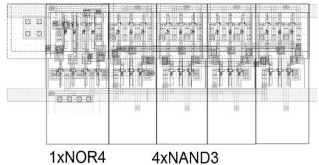
Figure 4: Pre-Decoder layout 1xNOR4 4xNAND3
