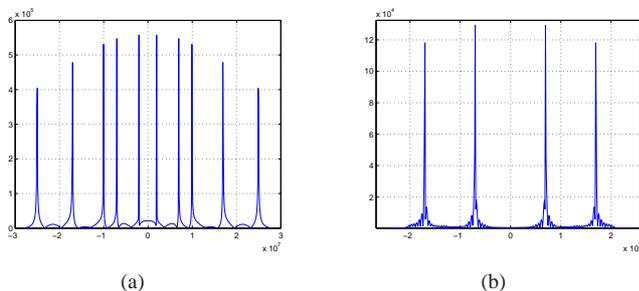
Fig. 5. (a) FFT of FIR filter input signal. (b) FFT of filtered signal.
