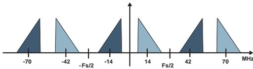
Fig. 3. Signal spectrum after sampling at 56 MHz.
