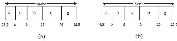
Fig. 2. Example of five bands of an GSM signal(a) Signal in FI. (b) Signal after undersampling
