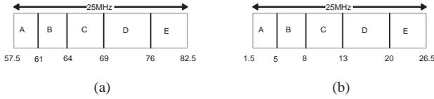
Fig. 2. Example of five bands of an GSM signal(a) Signal in FI. (b) Signal after undersampling
