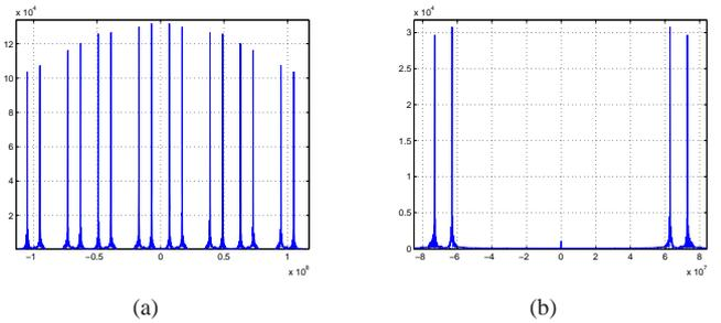
Fig. 6. (a) FFT of upsampled signal. (b) FFT of the recovered signal.
