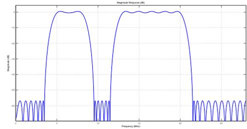
Fig. 4. Multiband FIR filter frequency response
