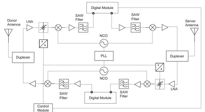
Fig. 1. Block diagram of a digital repeater.
