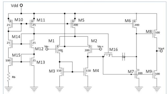
Figure 1: Three-stage opamp schematic.
