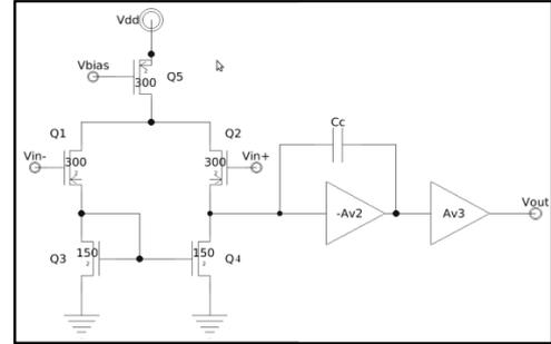
Figure 2: Compensation analysis equivalent circuit.
