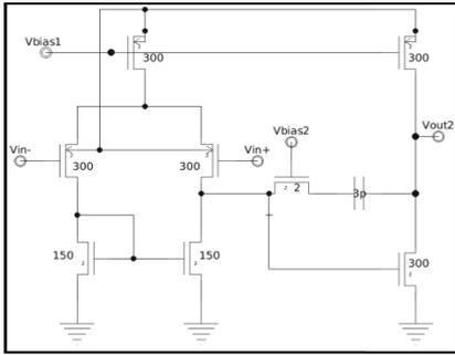
Figure 3: Equivalent circuit to frequency analysis.
