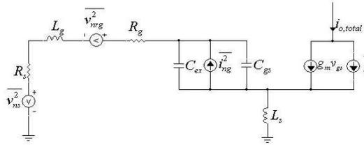
Figure 2. Small-signal model used to derive noise figure expression.
