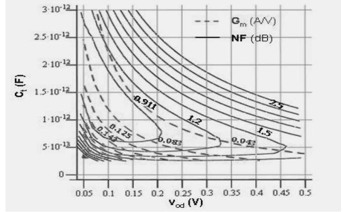
Figure 3. Overlaid plots of noise figure and transconductance (gain) for constante power consumption. Parameter used were:  $\gamma = 2/3$ ,  $\delta = 4/3$ ,  $c = j0.395$ ,  $E_{sat} = 4.7 \cdot 10^6$  V/m,  $v_{sat} = 8,43 \cdot 10^4$  m/s,  $f = 2.5$  GHz,  $P_D = 15$  mW,  $V_{dd} = 1.8$  V,  $R_{sheet} = 10$   $\Omega$ /square,  $W_f = 2.5$   $\mu$ m,  $Q_{ind} = 10$ ,  $L_{g,bw} = 1$  nH,  $Q_{ind,bw} = 50$  and  $Leff = 0.16$   $\mu$ m (0.18  $\mu$ m process).
