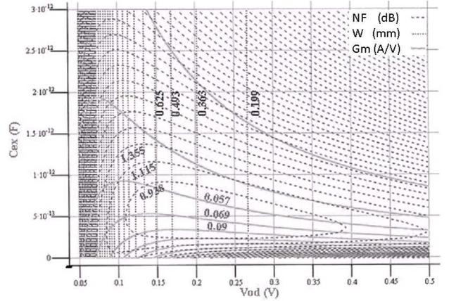
Figure 4. Overlaid plots of noise figure, tranconductance (gain) and transistor's length for constante power consumption. Parameter used were:  $\gamma = 2$ ,  $\delta = 4$ ,  $c = j0.395$ ,  $E_{sat} = 4.7 \cdot 10^6$  V/m,  $v_{sat} = 8,43 \cdot 10^4$  m/s,  $f = 0.915$  GHz,  $P_D = 4$  mW,  $V_{dd} = 1.8$  V,  $R_{sheet} = 8 \Omega/\text{square}$ ,  $W_f = 10 \mu\text{m}$ ,  $Q_{ind} = 100$ ,  $L_{g,bw} = 0$  nH,  $Q_{ind,bw} = 0$  and  $Le_{ff} = 0.29 \mu\text{m}$  (0.35 μm process).
