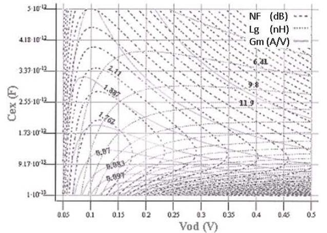
Figure 5. Overlaid plots of noise figure, tranconductance (gain) and inductor's size for constante power consumption. Parameter used were:  $\gamma = 2$ ,  $\delta = 4$ ,  $c = j0.395$ ,  $E_{sat} = 4.7 \cdot 10^6$  V/m,  $v_{sat} = 8,43 \cdot 10^4$  m/s,  $f = 0.915$  GHz,  $P_D = 15$  mW,  $V_{dd} = 1.8$  V,  $R_{sheet} = 8 \Omega/\text{square}$ ,  $W_f = 10 \mu\text{m}$ ,  $Q_{ind} = 4$ ,  $L_{g,bw} = 0$  nH,  $Q_{ind,bw} = 0$  and  $Le_{ff} = 0.29 \mu\text{m}$  (0.35 μm process).
