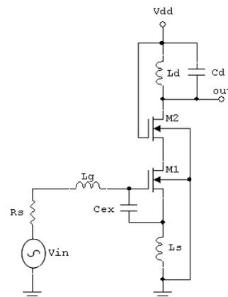
Figure 1. Inductively source-degenerated cascode adopted topology.
