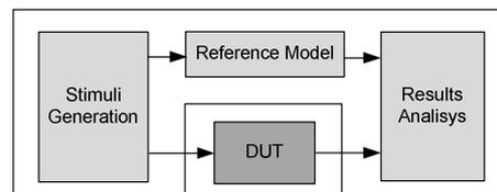
Figure 2. A self-checking testbench.
