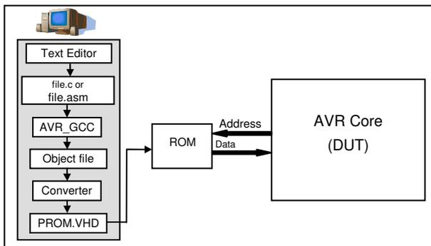
Figure 4. Initial test setup (without the proposed method).
