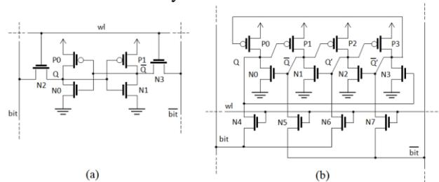
Figure 1. SRAM memory cells.
