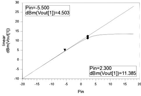
Fig. 5. Power gain versus input power in high gain mode
