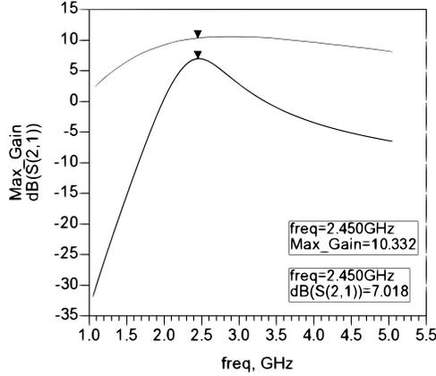
Fig. 6. Forward transmission gain  $S_{21}$  in low gain mode
