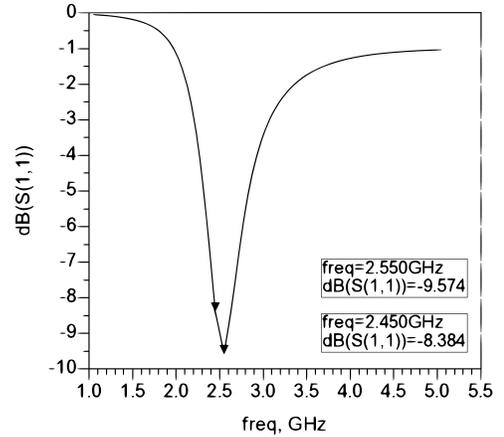
Fig. 4. Input reflexion coefficient  $S_{11}$
