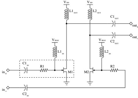
Fig. 1. Schematic of the pre-power amplifier
