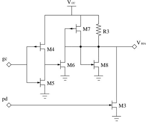
Fig. 2. Schematic of the biasing voltage generator
