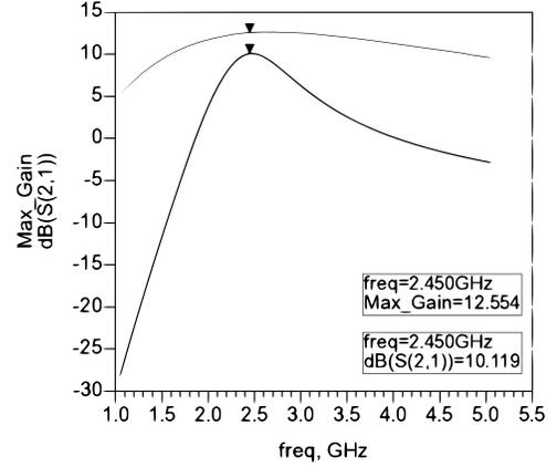
Fig. 3. Forward transmission gain  $S_{21}$  in high gain mode
