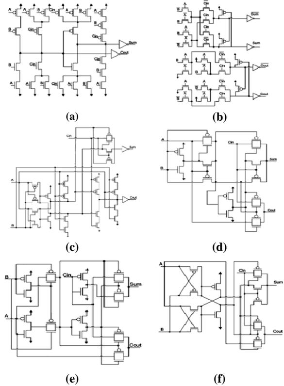
Figure 1 – Full-adder cells of different topologies [11]
