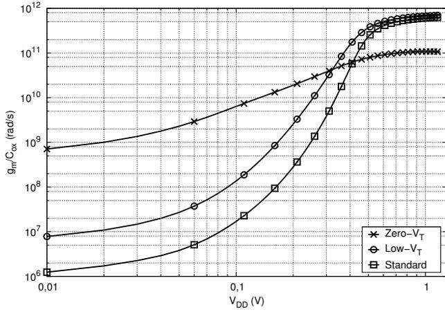
Fig. 2. Transconductance-to-capacitance ratio of the standard ( $W/L = 0.84\mu\text{m} / 0.12\mu\text{m}$ ), low- $V_T$  ( $W/L = 0.84\mu\text{m} / 0.12\mu\text{m}$ ) and zero- $V_T$  ( $W/L = 3\mu\text{m} / 0.42\mu\text{m}$ ) transistors. The transconductance  $g_m$  was simulated for  $V_S = V_B = 0$ , and  $V_D = V_G = V_{DD}$ .
