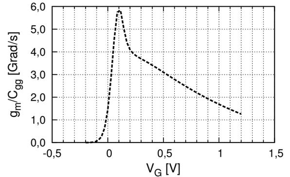
Fig. 9. The intrinsic transition frequency  $f_T$ .
