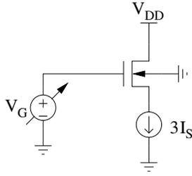
Fig. 10. Circuit used to extract the slope factor.
