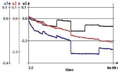
**Figure 5: Hamming network at 300 K: loss of functionality with noise of 46% of  $e$ .**
