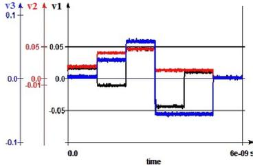
**Figure 4: Hamming network at 300 K: well characterized operation with noise of 45% of  $e$ .**
