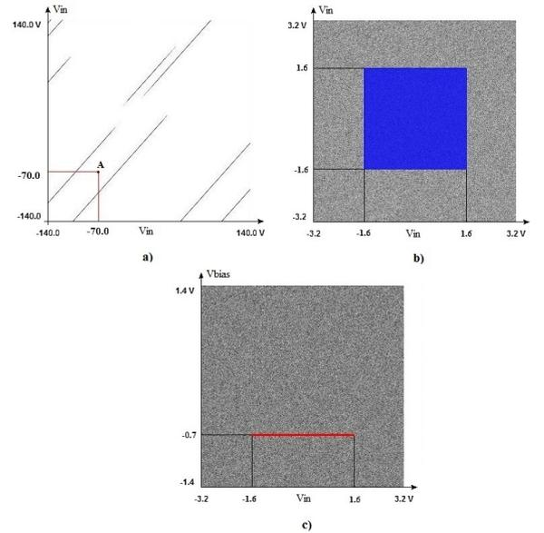
**Figure 3: All plots at 300 K. a) Hopfield stability plot. b) Hamming stability plot -  $V_{in}$  versus  $V_{in}$ . c) Hamming stability plot -  $V_{bias}$  versus  $V_{in}$ .**
