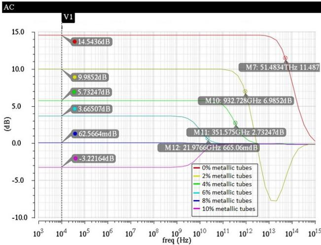
Fig. 4: Maximum voltage gain  $A_v$  as function of AC frequency. The gain of an ideal CNTFET remains stable even beyond the transit frequency of the transistor. The gain of CNTFETs with metallic tubes degrade before reaching the transit frequency.
