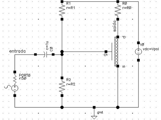
Fig. 3: Common-source CNTFET amplifier circuit.
