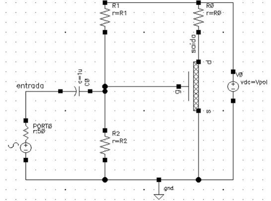
Fig. 3: Common-source CNTFET amplifier circuit.
