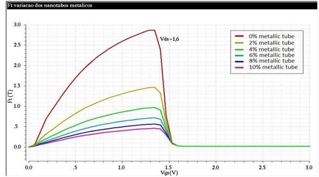
Fig. 1: Transition frequency ( $f_T$ ) versus  $V_{gs}$ , the employed drain bias is  $V_{ds} = 1.63$  V.
