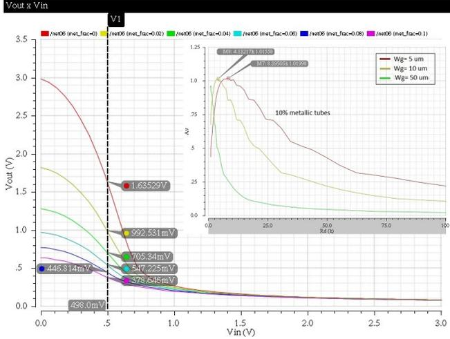
Fig. 2: Voltage transfer curve  $V_{out}$  ( $= V_{ds}$ ) vs.  $V_{in}$  ( $= V_{gs}$ ) for a drain resistance of  $R_0 = 10$  k $\Omega$  and CNTFETs with various metallic tube fractions. Inset: Maximum voltage gain  $A_v$  as function of the drain resistance  $R_0$  for a CNTFET with a fraction of metallic tubes of  $m_f = 0.1$ .
