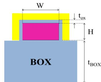
**Figure 2 –Front view of Junctionless SOI nMOSFET.**
