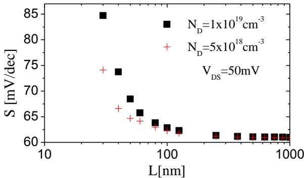
**Figure 5 – S versus L results for JNTs with L from 30 to 1000nm,  $N_D$  of  $1 \times 10^{19} \text{cm}^{-3}$  and  $5 \times 10^{18} \text{cm}^{-3}$  and  $V_{DS}=50\text{mV}$ .**
