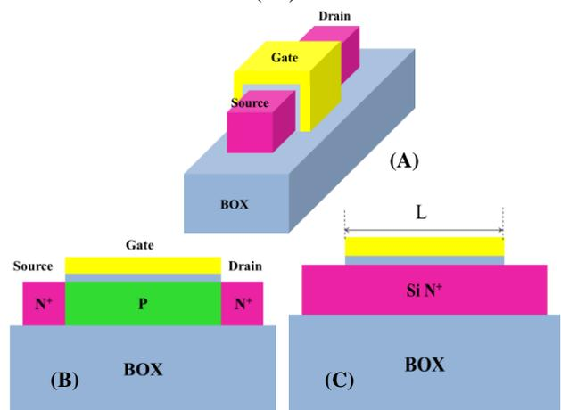
**Figure 1 – Standard (IM) and JNT perspective (A) and Standard (IM) (B) and JNT (C) SOI cross-section.**
