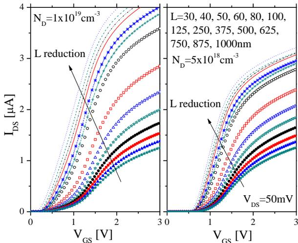
**Figure 3 –  $I_{DS}$  versus  $V_{GS}$  curves for JNTs with L from 30 to 1000nm,  $N_D$  of  $1 \times 10^{19} cm^{-3}$  and  $5 \times 10^{18} cm^{-3}$  and  $V_{DS}=50mV$ .**
