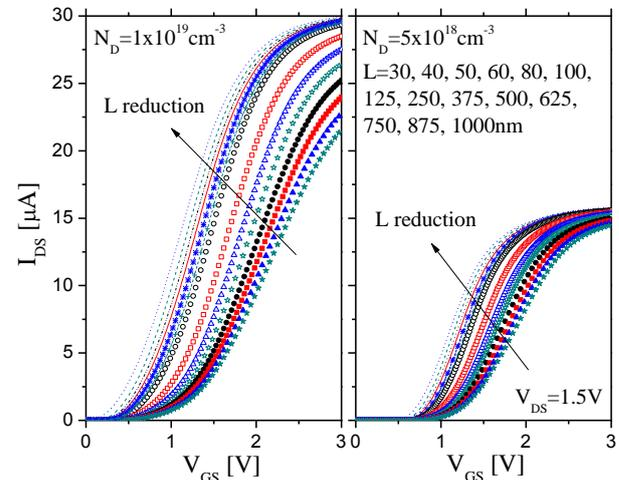
**Figure 7 –  $I_{DS}$  versus  $V_{GS}$  curves for JNTs with L from 30 to 1000nm,  $N_D$  of  $1 \times 10^{19} \text{cm}^{-3}$  and  $5 \times 10^{18} \text{cm}^{-3}$  and  $V_{DS}=1.5\text{V}$ .**
