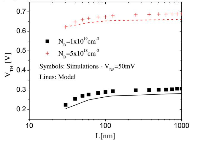
**Figure 4 –  $V_{TH}$  versus L results for simulations and model of JNTs with  $N_D$  of  $1 \times 10^{19} cm^{-3}$  and  $5 \times 10^{18} cm^{-3}$ .**
