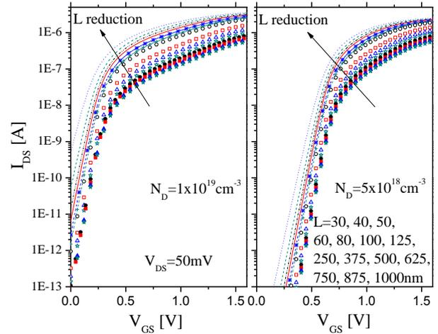
**Figure 6 – Logarithmic scale  $I_{DS}$  versus  $V_{GS}$  curves for JNTs with  $N_D$  of  $1 \times 10^{19} \text{cm}^{-3}$  and  $5 \times 10^{18} \text{cm}^{-3}$  and  $V_{DS}=50\text{mV}$ .**
