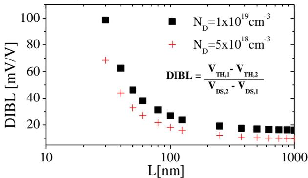
Figure 8 – DIBL versus L results for JNTs with L from 30 to 1000nm,  $N_D$  of  $1 \times 10^{19} \text{cm}^{-3}$  and  $5 \times 10^{18} \text{cm}^{-3}$ .
