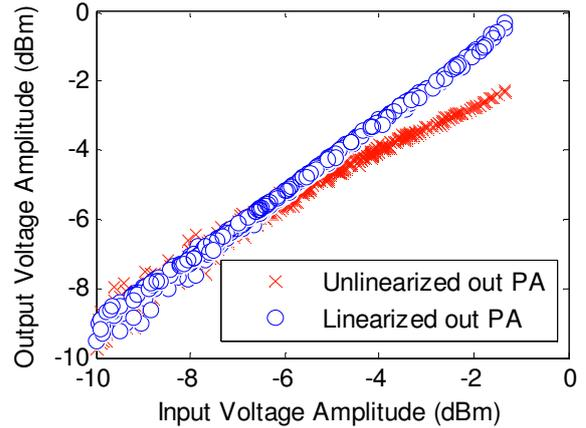
Figure 7. AM-AM plot of unlinearized and linearized PA, when  $R = 25$  and the number of bits used for the representation of the binary numbers is set to 22.
