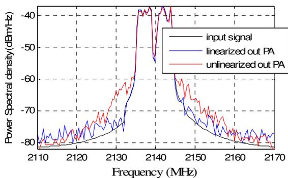
**Figure 8. Power Spectral Density, when  $R = 25$  and the number of bits used for the representation of the binary numbers is set to 18.**
