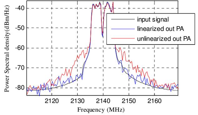
Figure 6. Power Spectral Density, when  $R = 25$  and the number of bits used for the representation of the binary numbers is set to 22.
