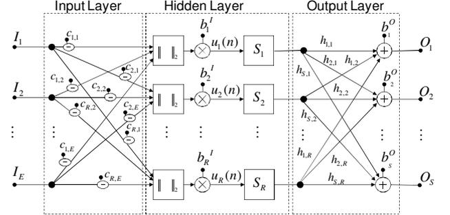
Figure 3. Block diagram of an RBF neural network.
