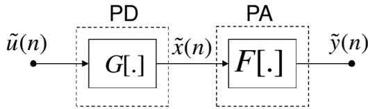
Figure 2. Cascade connection of a PD followed by a PA.
