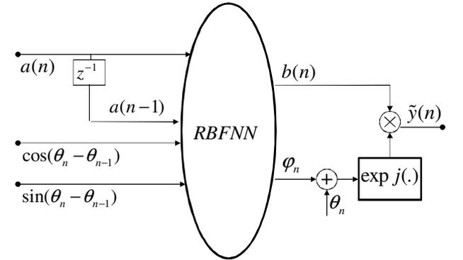
Figure 4. Block diagram of an RBFNN DPD having  $M = 1$ .
