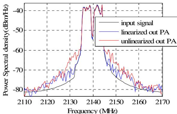
**Figure 9. Power Spectral Density, when  $R = 20$  and the number of bits used for the representation of the binary numbers is set to 22.**
