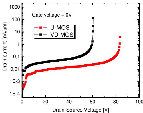
**Figure 7 – Simulated breakdown characteristics.**
