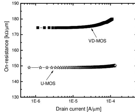
Figure 4 – On-resistance behavior for the different power MOS transistors.
