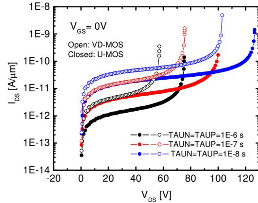
**Figure 8 – Simulated breakdown characteristics for different lifetime.**
