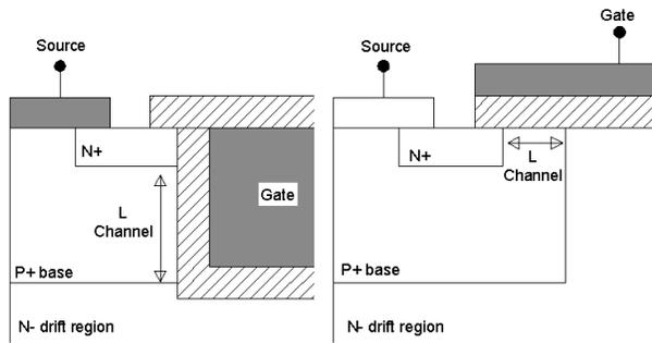
Figure 3 – Schematic cross-section of a (a) U-MOS and (b) VD-MOS power transistors indicating the channel length.
