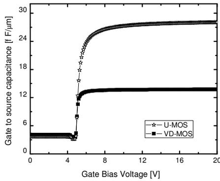
Figure 2 – Gate capacitance behavior for the different power MOS transistors.
