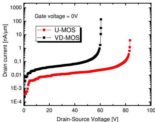
**Figure 7 – Simulated breakdown characteristics.**
