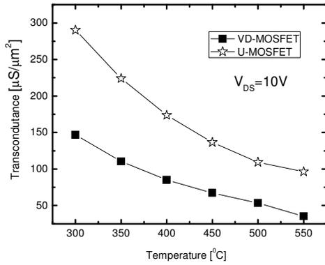
**Figure 6 – Transconductance extracted for the different power MOSFET structures as a function of the temperature.**
