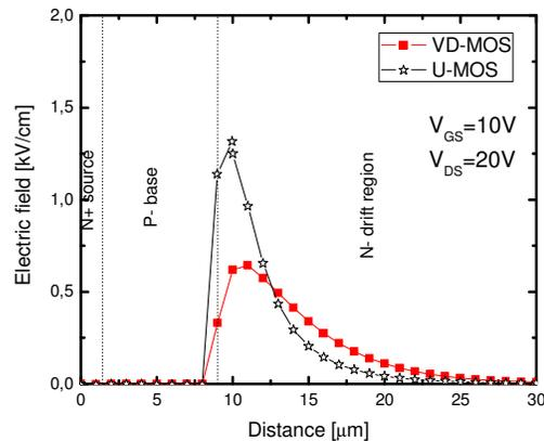
**Figure 9 – Simulated electric field for the different MOS structures.**
