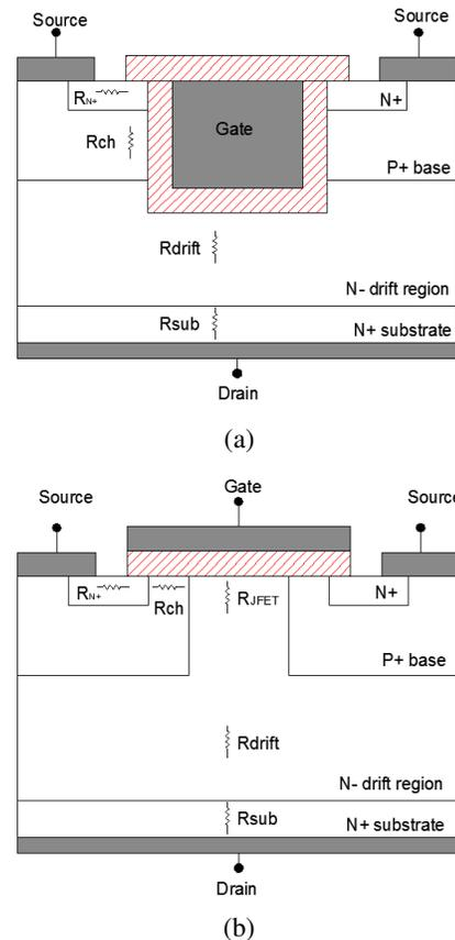
Figure 5 – Schematic cross-section of a (a) U-MOS and (b) VD-MOS power transistors indicating all the resistance components.
