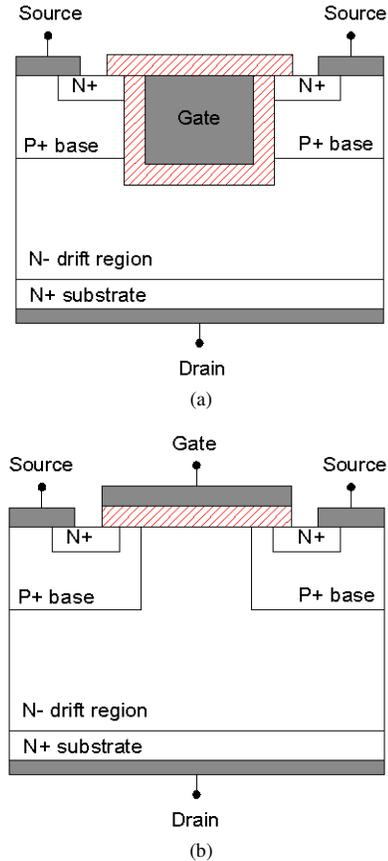
Figure 1 – Schematic cross-section of a (a) U-MOS and (b) VD-MOS power transistors.
