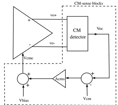
**Figure 2: Conceptual Common-Mode Feedback block [6].**
