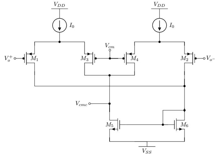
**Figure 4: Common-mode Feedback Circuit.**
