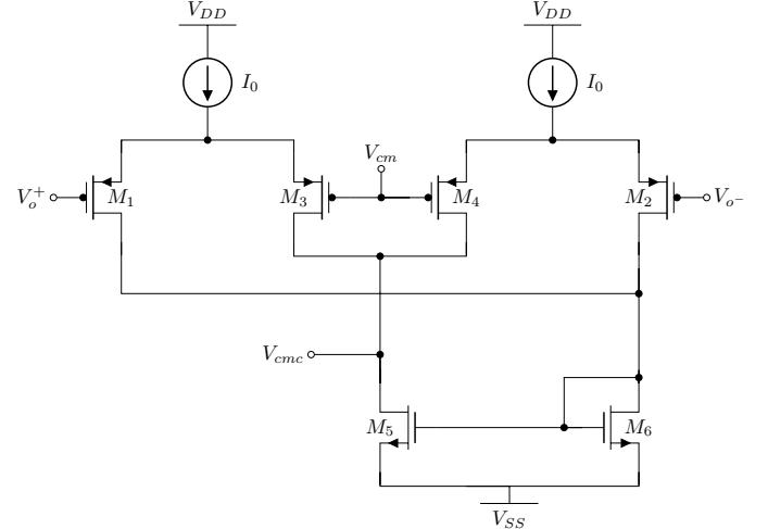
**Figure 4:** Common-mode Feedback Circuit.
