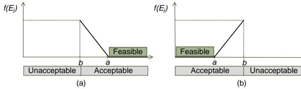
**Figure 1: Cost function performance metric, (a) minimum required value specifications and (b) maximum required value specifications.**
