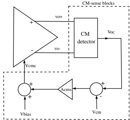
**Figure 2: Conceptual Common-Mode Feedback block [6].**
