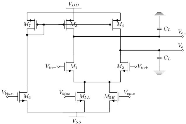
**Figure 3: Schematics of a single-stage fully differential amplifier circuit.**
