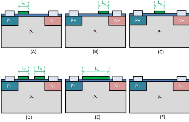
Figure 2. (A) Offset left: device with the gate adjacent to P+ region. (B) Offset right: device with gate adjacent to N+ region. (C) Central gate: gate in the middle of the device. (D) Dual gate: device with simultaneous right gate and left gate. (E) Full gate: gate all over the entire intrinsic region. (F) No gate: common lateral PIN photodiode, with no gate.
