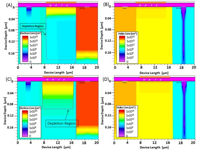
Figure 3. Cross-section of a photodiode structure showing electrons concentration for positive  $V_G$ , and holes concentration for negative  $V_G$  for (A) Offset right device with  $V_G = +3V$ . (B) Offset left device with  $V_G = -3V$ . (C) Central gate device with  $V_G = +3V$ . (D) Central gate with  $V_G = -3V$ . All the structures are under light incidence of wavelength ( $\lambda$ ) of  $637\text{nm}$ .
