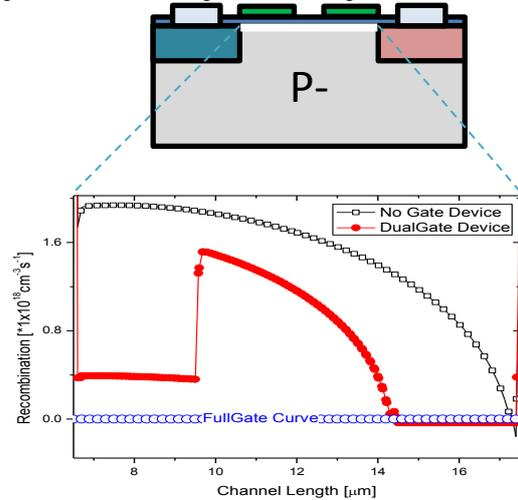
Figure 9. Recombination rate as a function of the device length. This plot was made considering a cross-section of the first interface through the channel.
