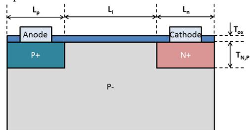
Figure 1. Cross-section of one finger of a PIN photodiode.
