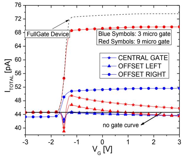
Figure 5. Photogenerated current ( $I_{TOTAL}$ ) as a function of the gate bias ( $V_G$ ), for different devices and gate sizes, with the ITO gate material for  $\lambda$  of 637nm.
