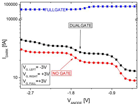
Figure 8. Dark current ( $I_{DARK}$ ) as a function of the anode bias for dual gate and no gate devices for ITO gate material.
