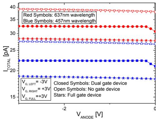
Figure 7. Photogenerated current as a function of the anode bias for dual gate ( $V_{G, LEFT} = -3V$  and  $V_{G, RIGHT} = +3V$ ), full gate ( $V_{G, FULL} = +3V$ ) and no gate device with aluminum gate material.
