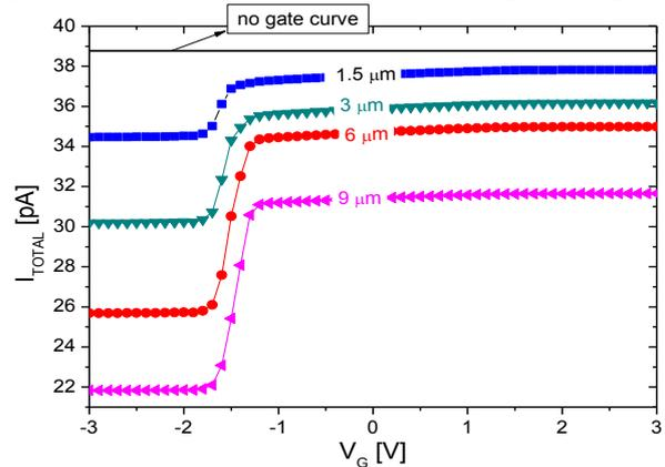
Figure 6. Photogenerated current as a function of the gate voltage ( $V_G$ ) for the offset right device with different gate lengths. (with gate material of aluminum) for  $\lambda$  of 637nm.
