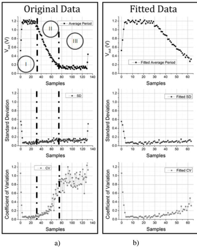
**Figure 4.** Chart representing the steps of the methodology. 4a. Samples studied in its original form. 4b. Samples studied after reducing the noise
