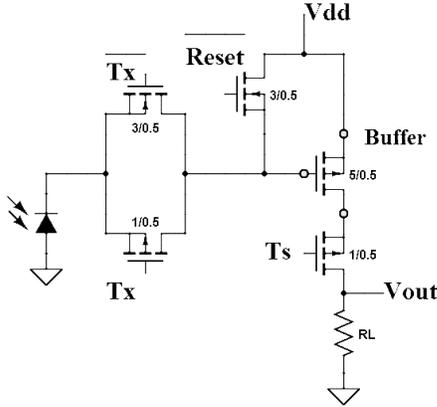
Figure 2. Basic diagram of the 4T APS
