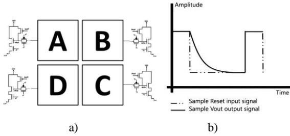
Figure 1. 1a Quad-cell representation with its electronic circuits. 1b Sample decay curve of a photodiode.
