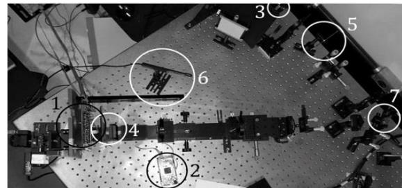
**Figure 5.** Optical table with the instruments and devices used for the experiment: 1-Chip’s *PCB*; 2-Arduino microcontroller board; 3-Laser source; 4-Etched glass; 5-Intensity filter; 6-Light power meter; 7-Beam splitter.
