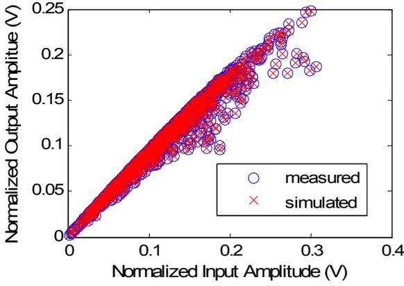
Figure 1. Output amplitude as a function of the input amplitude for the WCDMA signal: measured at the DBPA and estimated by the Volterra series of (4).
