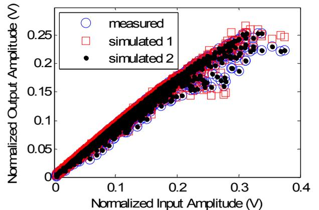
Figure 4. Output amplitude as a function of the input amplitude for the OFDMA signal: measured at the DBPA and estimated by the original Volterra series of (4) and by the modified Volterra series of (4) that includes additional terms.
