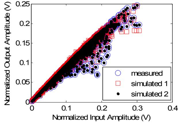
Figure 3. Output amplitude as a function of the input amplitude for the WCDMA signal: measured at the DBPA and estimated by the original Volterra series of (4) and by the modified Volterra series of (4) that includes additional terms.
