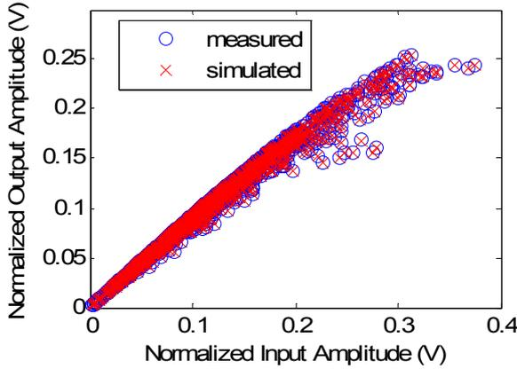
Figure 2. Output amplitude as a function of the input amplitude for the OFDMA signal: measured at the DBPA and estimated by the Volterra series of (4).
