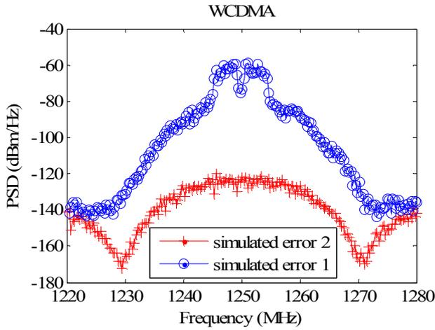
Figure 5. PSDs of the error signals for the WCDMA signal: simulated error 1 uses the original Volterra series of (4); simulated error 2 uses the modified Volterra series of (4) that includes additional terms.
