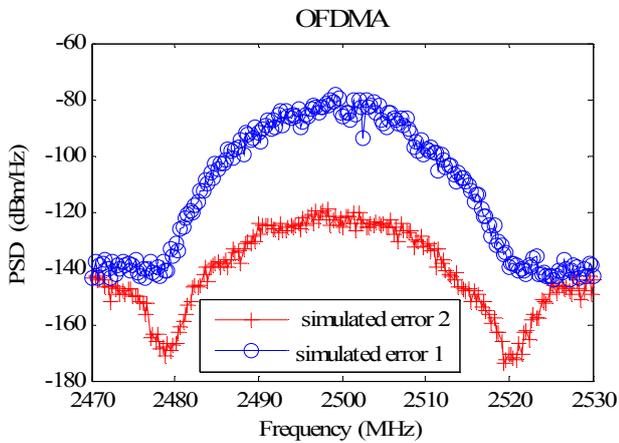
Figure 6. PSDs of the error signals for the OFDMA signal: simulated error 1 uses the original Volterra series of (4); simulated error 2 uses the modified Volterra series of (4) that includes additional terms.
