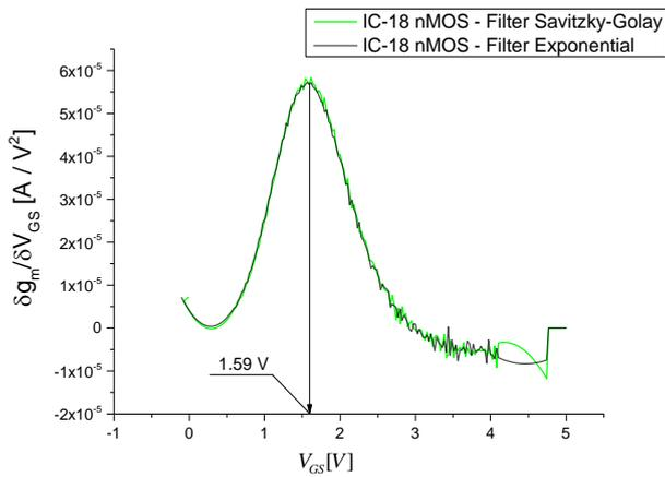
Fig.5.  $\partial g_m/\partial V_{GS}$  curve IC-18 compared for nMOS device.
