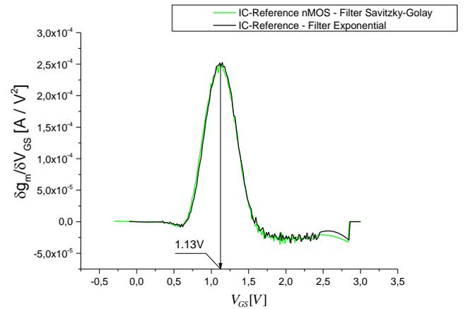
**Fig.1.**  $\partial g_m / \partial V_{GS}$  curve for IC-Reference nMOS device.
