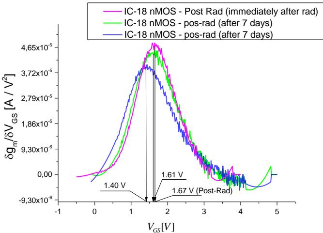
**Fig.3.**  $\delta g_m / \delta V_{GS}$  curve IC-18 compared for nMOS device.
