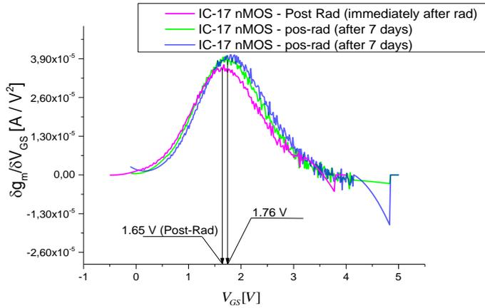
**Fig.2.**  $\delta g_m / \delta V_{GS}$  as a function of the  $V_{GS}$  for DUT IC-1, after 3 Mrad..
