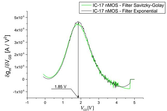
**Fig.4.**  $\delta g_m / \delta V_{GS}$  curve IC-17 compared for nMOS device.
