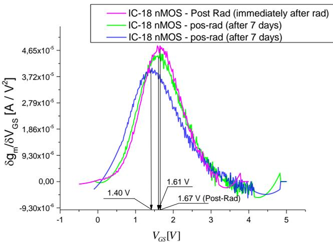
**Fig.3.**  $\delta g_m / \delta V_{GS}$  curve IC-18 compared for nMOS device.
