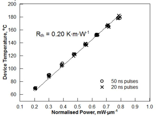
Fig. 3. Device temperature as function of the normalized power to obtain the thermal resistance. Source: [3].
