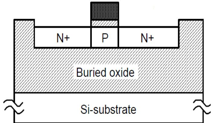
Fig. 1. The SOI transistor. Source: [5]
